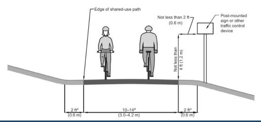
Typical Cross Section of Two-Way, Shared Use Path on Independent Right-of-Way (Figure 5-2, AASHTO Guide for the Development of Bicycle Facilities, 2012)
