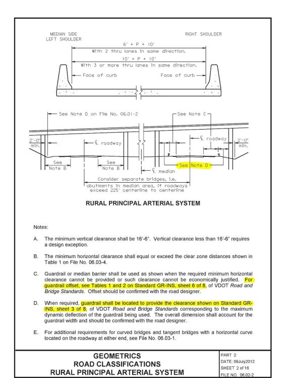
Figure 14 – VDOT requirements for clear zones
