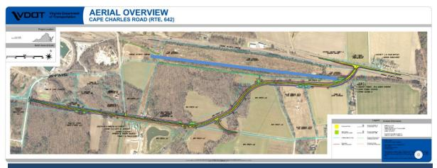
**Figure 3** - Improvements to Route 642 include 4' paved shoulders but no standalone trail option. The blue line shows temporary drainage easements that may be attractive alianments for Phase IV of the trail.
