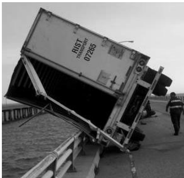
FIGURE 19.7 Sudden high winds created by a suspected microburst overturned two trucks on the Chesapeake Bay Bridge Tunnel in May 2011. One of the overturned trucks is shown. Photo from Eastern Shore News.
